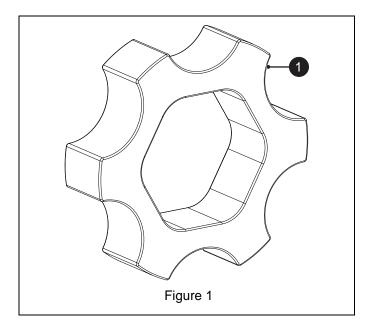
3. Align rubber grip ring (item 1) to drive control grip and push onto drive grip until fully seated. See Figure 2.
