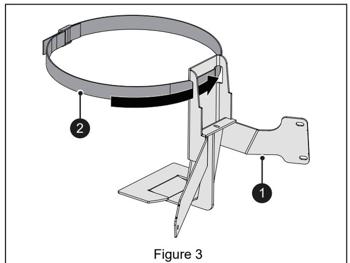
2. Install bucket mounting assembly to right fender and secure with tapping screws removed earlier. See Figure 4.
